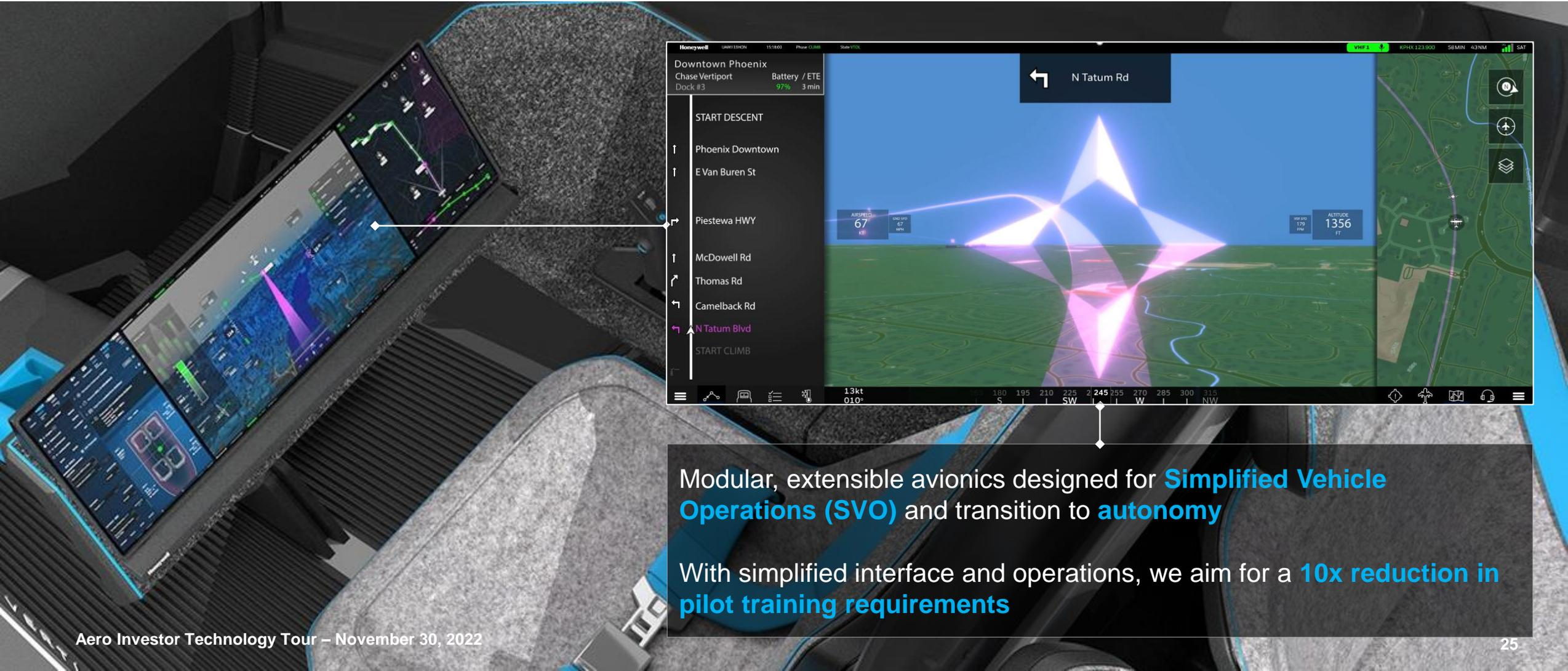
Modular, extensible avionics designed for **Simplified Vehicle Operations (SVO)** and transition to **autonomy**
