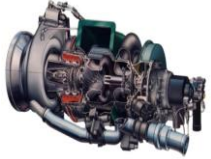
Auxiliary Power Unit
